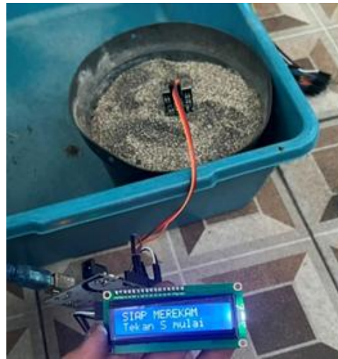
Figure 1. Experimental configuration of the Arduino-based soil moisture monitoring system using Regosol. Source: research documentation, 2026.
