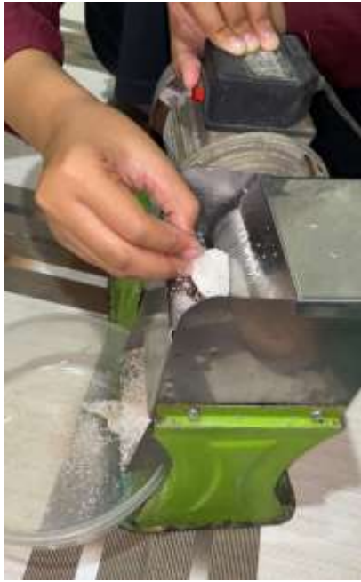
Figure 1. Grating of coconut flesh as part of the VCO production process.
